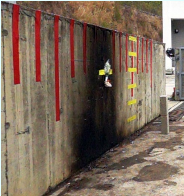
Figure 1) Moment of impact: glass broke scattering liquid
