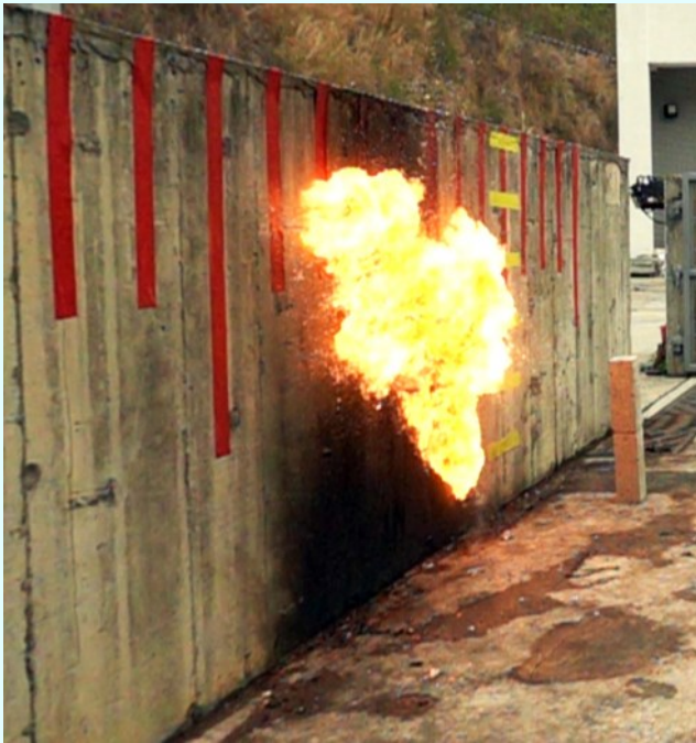
Figure 5) 80 ms post-impact: ~1.5m diameter fire ball had developed
