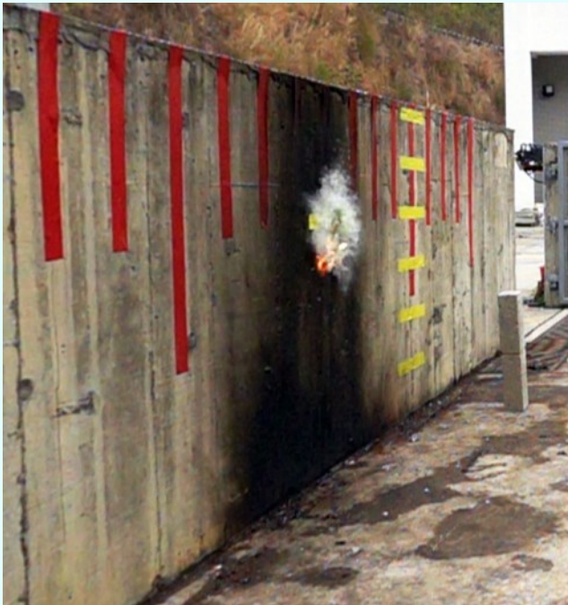
Figure 2) 10 ms post-impact: liquid scattered but fire yet to develop
