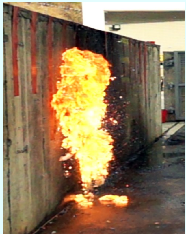
Figure 8) 150 ms post-impact: fire development with cooking oil/petrol at ratio of 1:1
