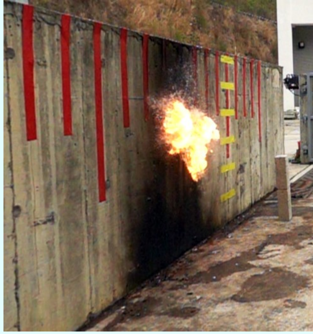
Figure 4) 40 ms post-impact: ~1m diameter fire ball had developed
