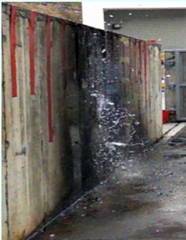
Figure 7) 150 ms post-impact: fire development with detergent/petrol at ratio of 1:1
