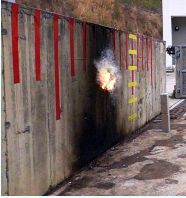
Figure 3) 20 ms post-impact: liquid scattered and fire began to develop
