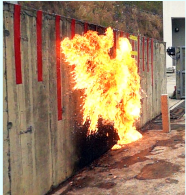
Figure 6) 150 ms post-impact: ~2m diameter fire ball had developed
